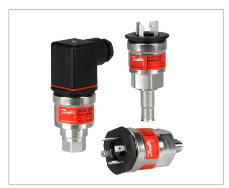
AKS 32R is a ratiometric pressure transmitter that converts the measured pressure to a linear output signal. The min. value of the output signal is less than 10% of the actual supply voltage. The max. value is more than 90% of the actual supply voltage.
